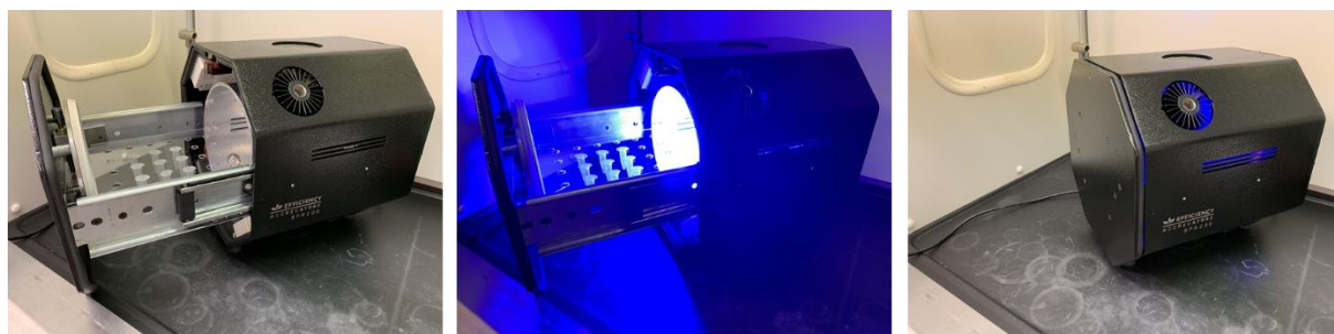
Supporting Figure 27. Left panel, bio-photoreactor (switched off) containing microcentrifuge tubes in sample rack. Middle panel, bio-photoreactor (switched on) with visible light irradiation at full intensity. Right panel, bio-photoreactor (switched on) in normal operating mode at full light intensity with chamber door closed.
