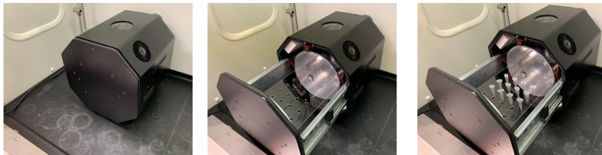
Supporting Figure 26. Left panel, bio-photoreactor (switched off), door closed. Middle panel, bio-photoreactor (switched off), door open. Right panel, bio-photoreactor (switched off), door open with Eppendorf tubes inserted.
