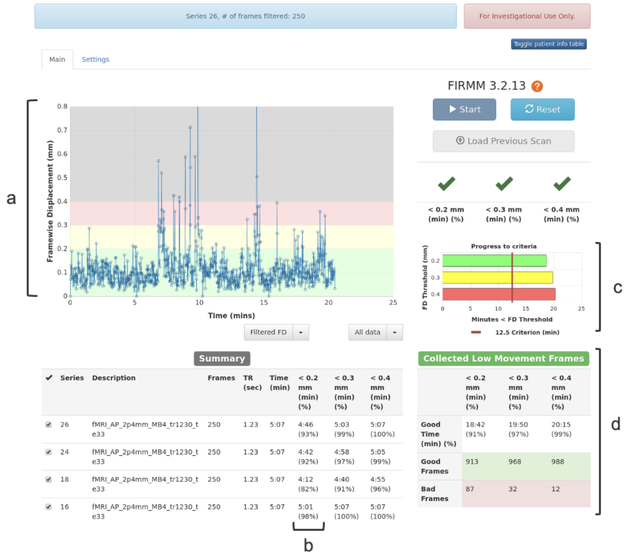
Figure 1. FIRMM Prototype software available in 2017 and used for data collection in Cohorts 4 and 5. (a) Motion Trace : plot of FD values for each frame (b) < 0.2 mm (min) (%): minutes and percentage of functional MRI data collected below 0.2 mm for a particular sequence; (c) Progress to criteria : total minutes of data collected compared to a predetermined minimum goal of low-motion data; and (d) Collected Low Movement Frames : running total of minutes, percent, and number of frames of usable data.
