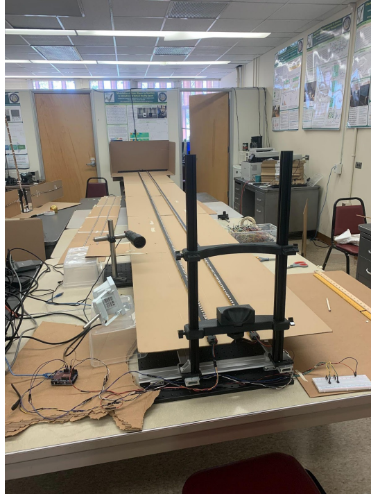
Figure 8. The 5m LED Depth Setup used at UCLA Knudsen Hall.
