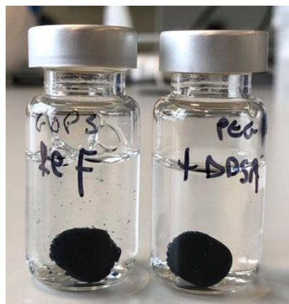
Figure S4: PEDOT:PSS-based scaffolds crosslinked with GOPS 3 wt% (right) and PEGDE 3 wt% (left) immersed in aqueous PBS 1X for more than 6 months.
