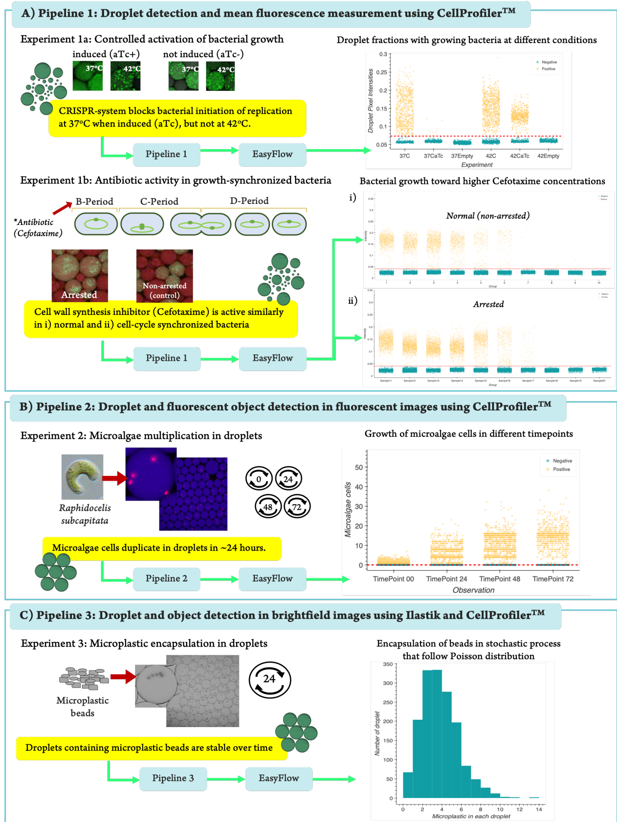
Figure 4. Demonstration of EasyFlow pipelines in experimental scenarios. A) Here, we show that bacteria growth can be controlled via temperature sensitive CRISPR system (Exp. 1a) and bacteria respond to antibiotics similarly regardless of their synchronization in cell cycle (Exp. 1b). B) Microalgae multiply in droplets stably over 72h incubation period (Exp 2). C) Microplastic beads do not affect the stability of droplets during 24h incubation (Exp. 3). In this figure, we show only one representative graph for each experiment. Full info for each experiment is added in the Supplementary Figure 6.
