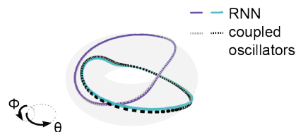
Fig S4. Converged RNN dynamics match those of coupled oscillators. We simulated two coupled oscillators with the coupling function extracted from a trained network (Fig. 3B). The two oscillators represent the RNN's phase ( \phi ) and the reference oscillation phase ( \theta ). Starting simulations from various initial conditions demonstrates that the coupling function induces bistability, as all simulations converge to one of two stable cycles on the torus. Furthermore, the convergent trajectories of the coupled oscillators are a close match to those of the full RNN projected into the same space ( \phi, \theta ), indicating that the coupled oscillator description is appropriate for the RNN.
