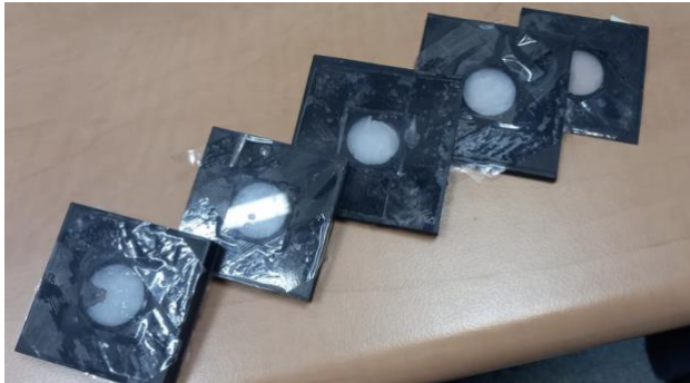
Figure S7: The sliced tissue-like phantoms were used for the FLI experiments. For each experiment, a slightly oversized slice of phantom was cut and placed on a phantom holder comprised of a glass coverslip bottom taped to the 3D printed spacer of appropriate thickness (0.1, 0.3, 0.5, 0.7 and 1 cm), then cut with a knife to achieve the desired thickness, and covered with another coverslip.
