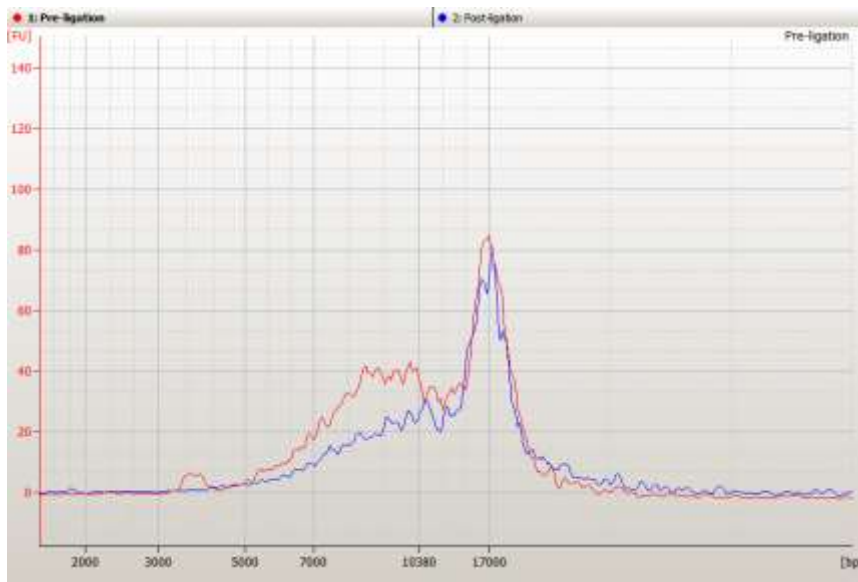
Figure S3A. Bioanalyzer traces prepared from an Oxford library sheared at 10kb before and after adapter ligation. The large peak at 17k is the upper marker.
