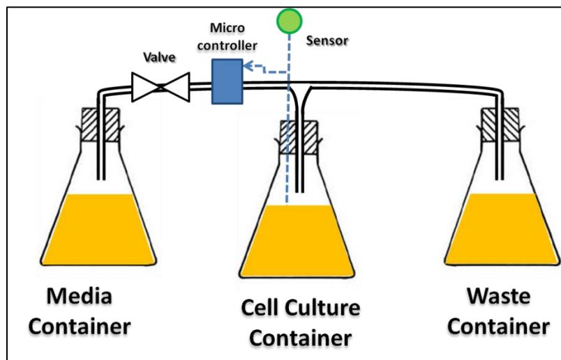
**Supplementary Figure 1:** A sketch of a Turbidostat- The liquid (media) flows from the media to the cell container and further into a waste container. The OD is measured using the sensor (green). The flow rate is controlled using the micro-controller which in turn controls the actuators like valves and pumps.
