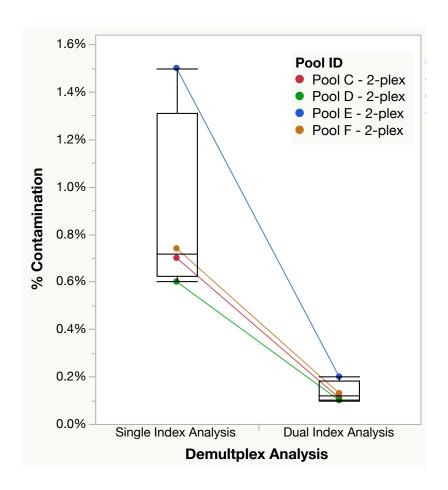
Supplemental Figure 1: Initial testing of single vs dual indexed sequencing on HiSeq. For four pools of 2 libraries, both the i7 and i5 indexes were read. Demultplexing was then performed two ways, once using just the i7 single index and again using both the i7 and i5 dual indexes. The % contamination rate decreased dramatically when dual indexing demultiplexing was performed.
